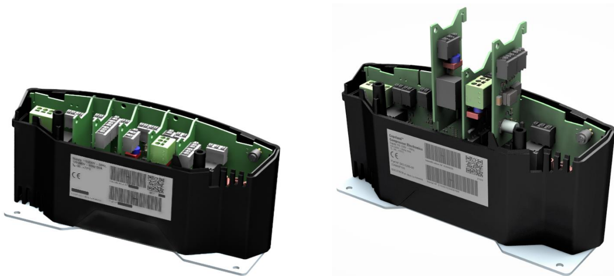
Figure 3: Inside view of the Copeland Compressor Electronics module, with the modular boards
