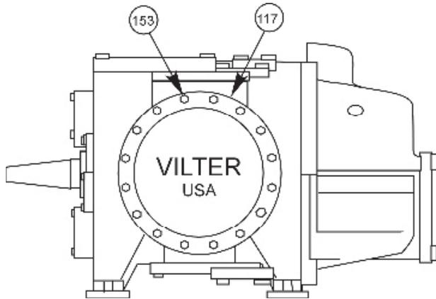
For VSM 451 thru 601 compressors, do not use side rails.
