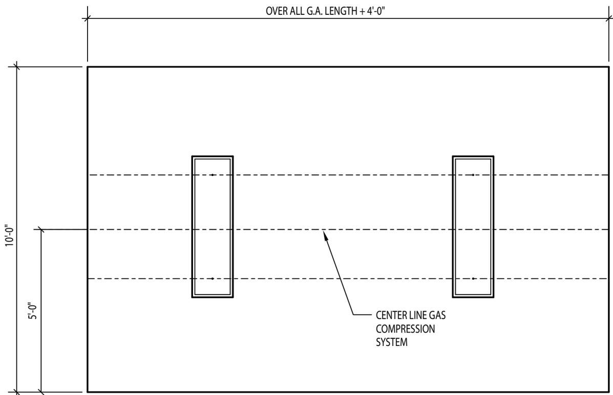
Figure 4. Foundation with Housekeeping Pads Dimensions - Top View
