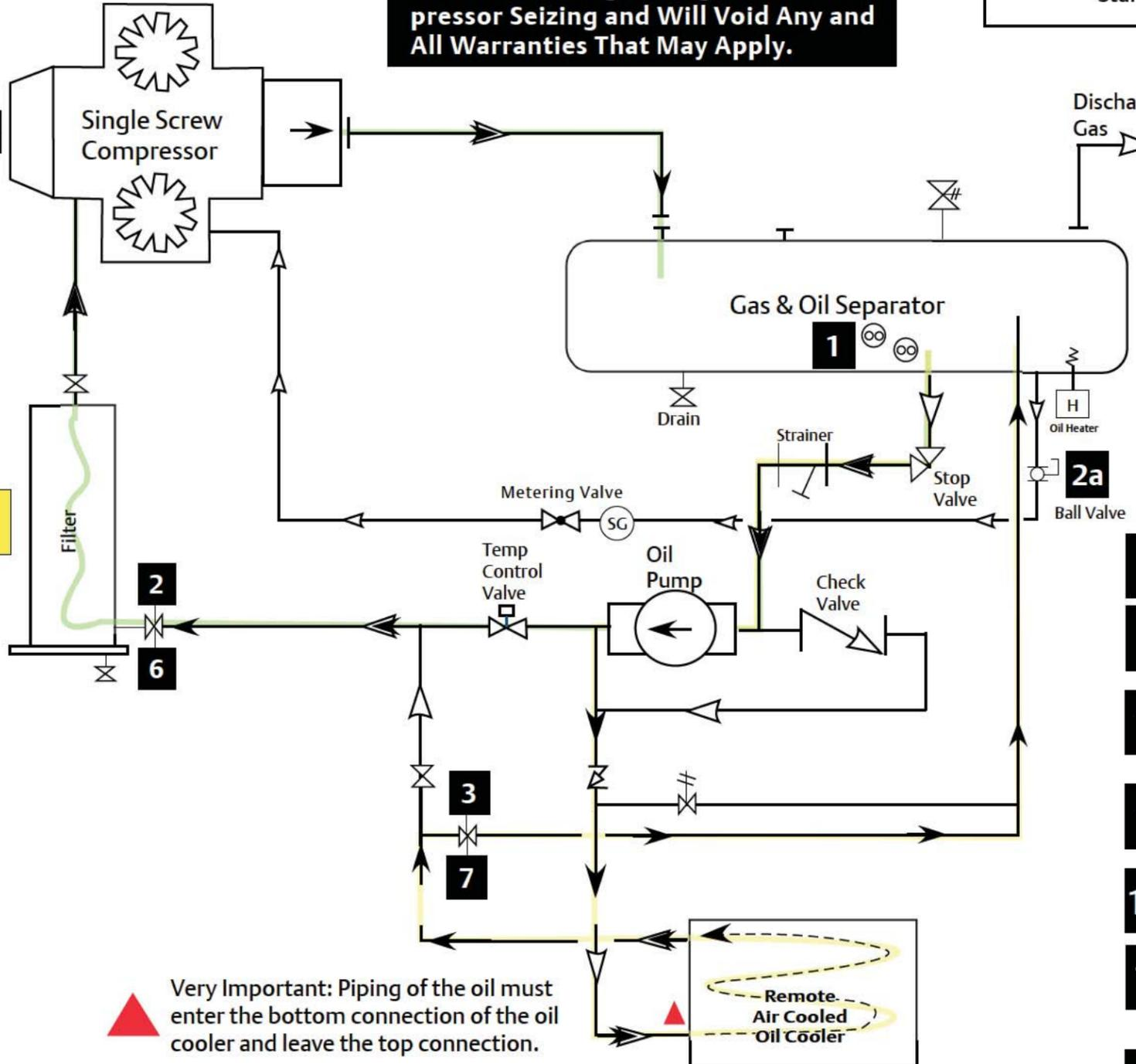
▲ Very Important: Piping of the oil must enter the bottom connection of the oil cooler and leave the top connection.
