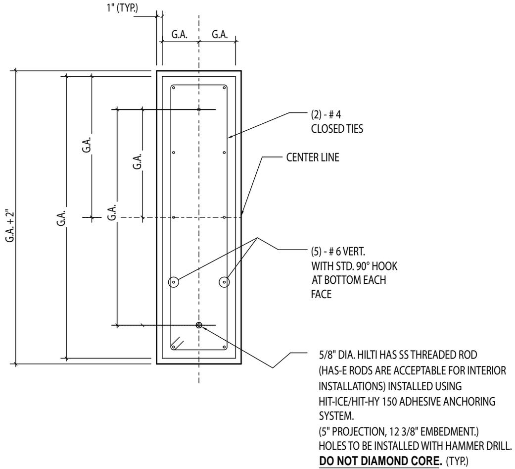
Figure 5. Housekeeping Pad Dimension Detail - Top View
