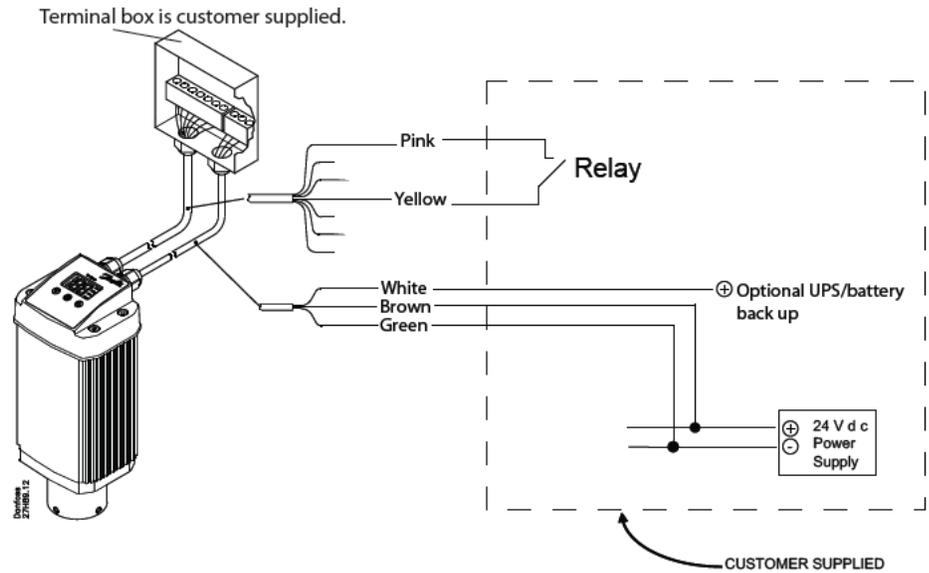
**Wiring diagram showing ICAD digital outputs wired with customer supplied auxiliary relays**
