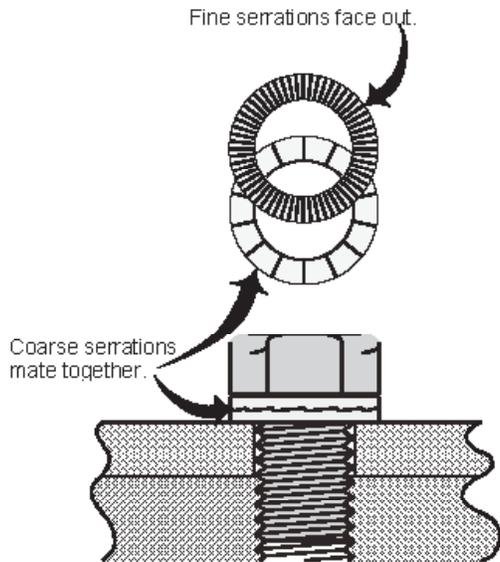
A. The Nord-Lock® lock washer sets are used in many areas in both the VSG & VSSG screw compressors that require a vibration proof lock washer.
