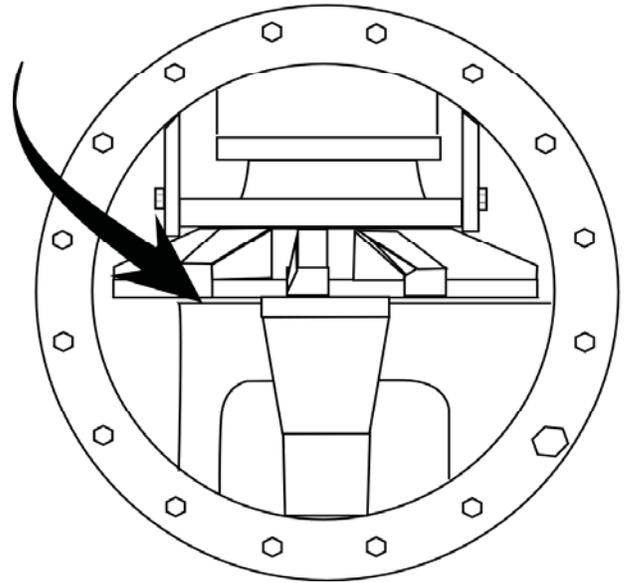
**Note:** Replacement blades are precisely the same dimensionally as blades installed originally at factory: Therefore, the same amount of shims will be required for replacement blades.
