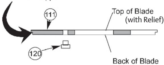
Snap ring bevel must be positioned away from the blade on gaterotor.
