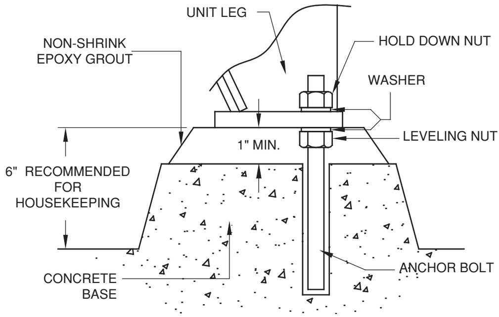
Figure 7. Concrete Pad Housekeeping Detail
