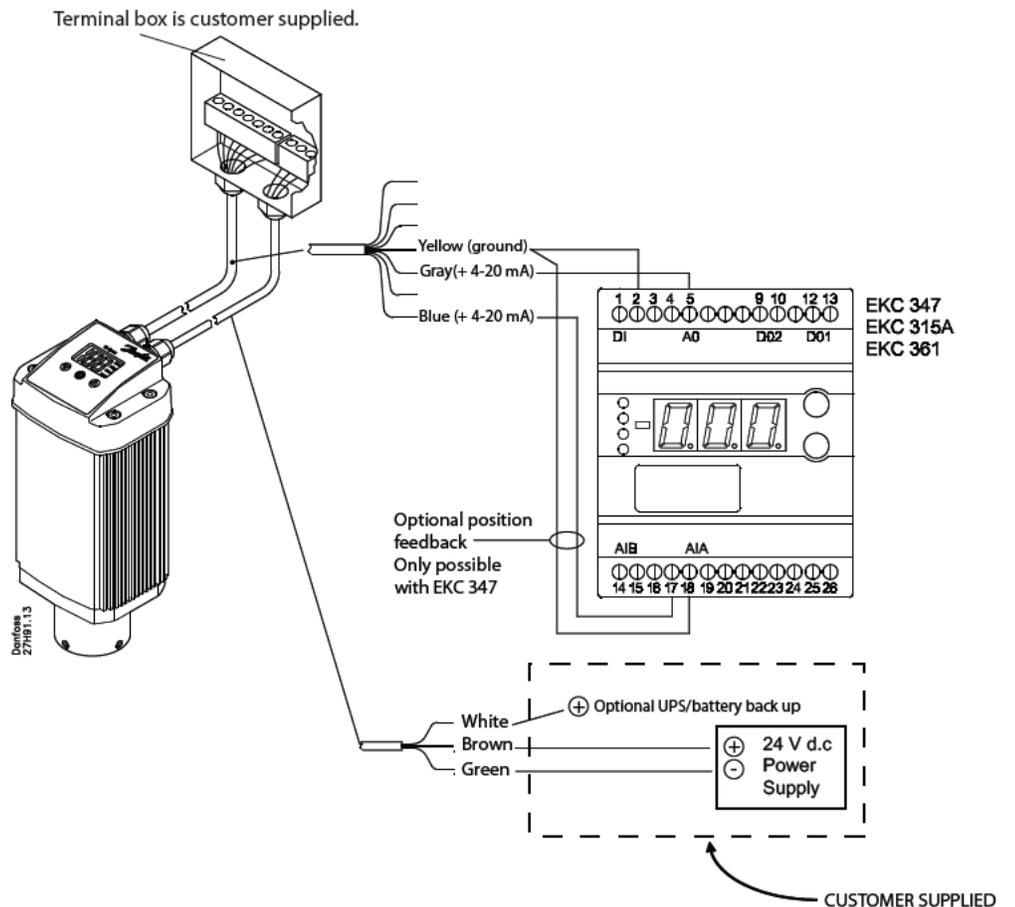
**Wiring diagram showing ICAD wired with a digital input for ON/OFF solenoid valve operation**
