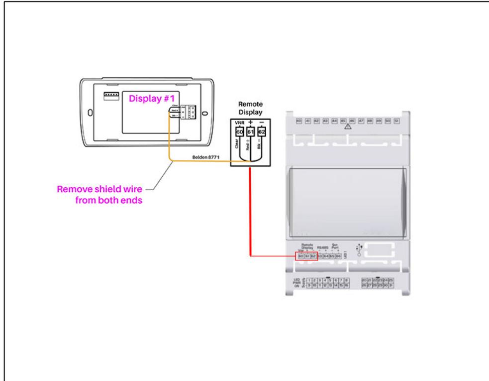
Figure 3-2 - Visograph connection
