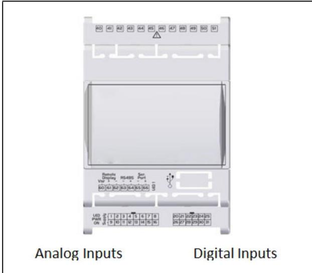
Figure 4-1 - Pump Skid Controller Input Locations
