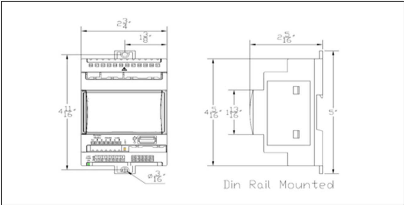
Figure 2-1 - DIN Mounting
