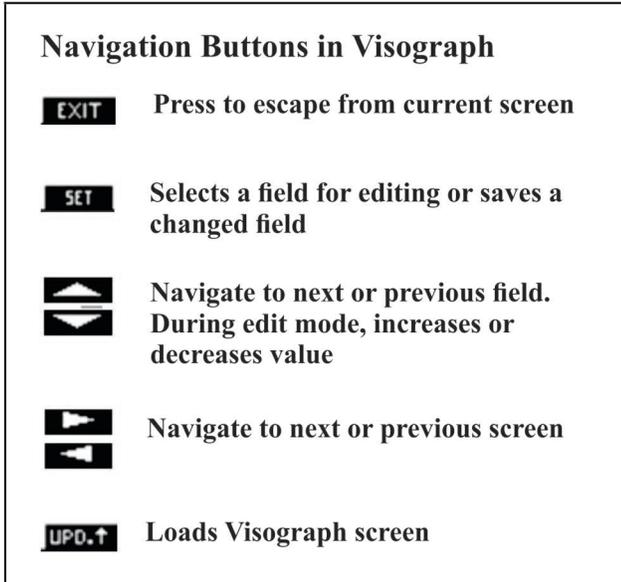
Figure 3-3- Visograph Buttons
