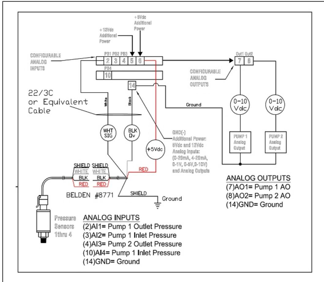
Figure 4-6 - Analog Output Wiring
