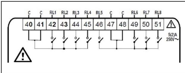
*Figure 4-5 - Relay Output Wiring*
