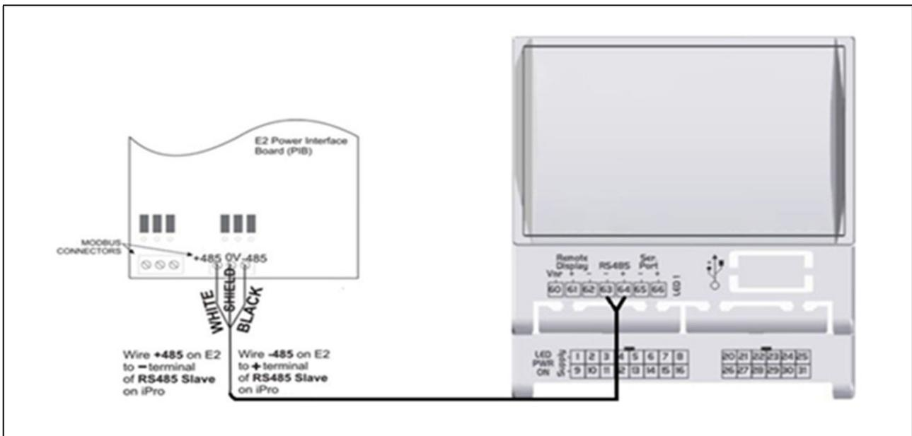
Figure 3-1 - MODBUS Networking
