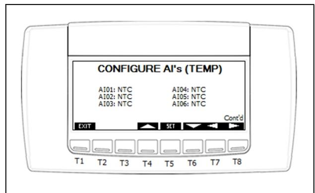
Figure 9-6 - Configure Analog Input's Temperature
