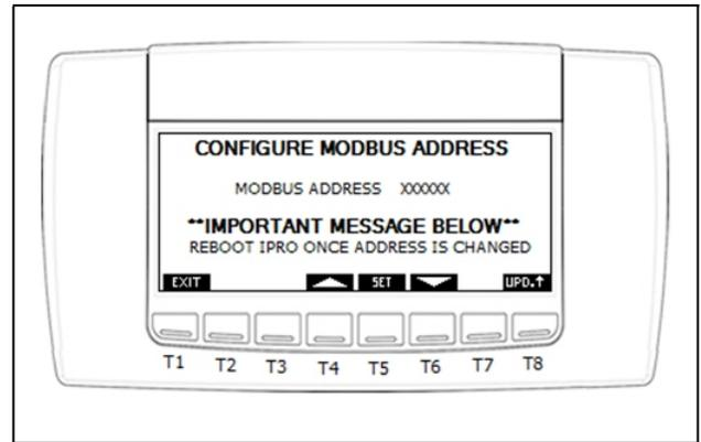
Figure 9-18 - Configure MODBUS Address
