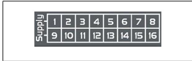
Figure 4-10 - Analog Output Connectors
