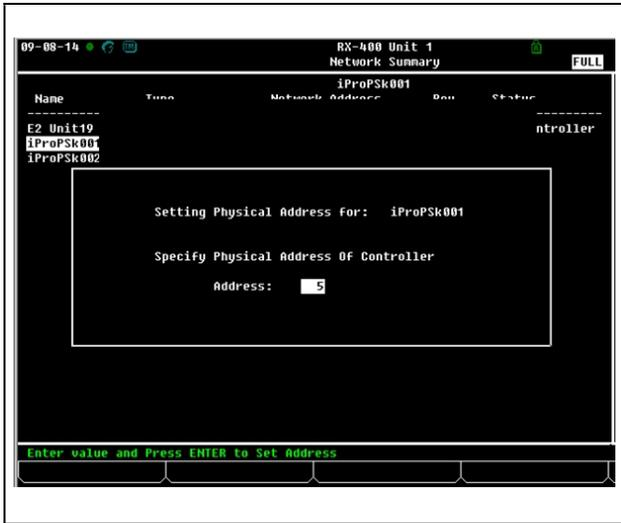
Figure 7-5 - Set the Address of the Pump Skid controller
