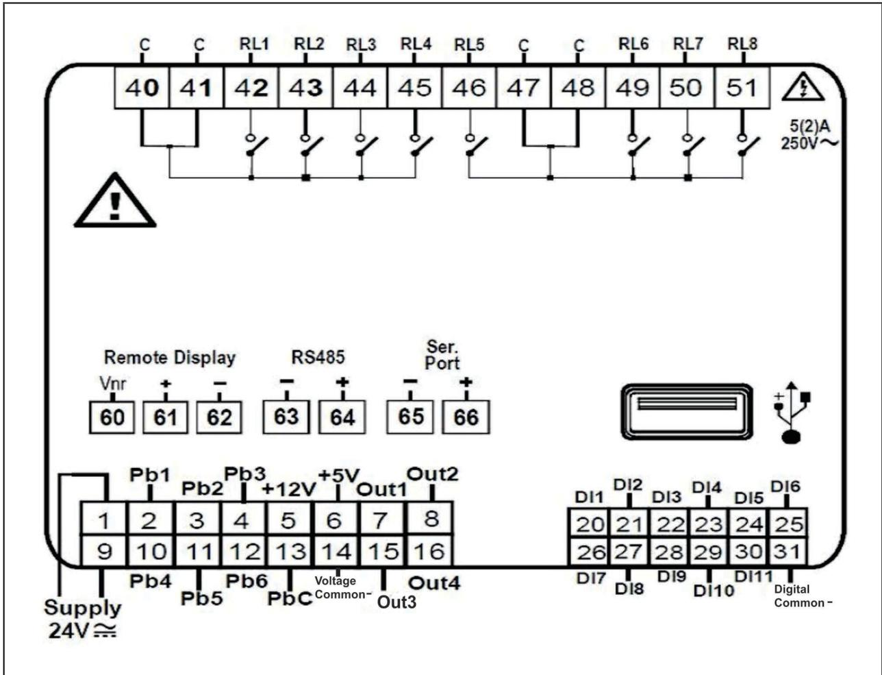
Figure 8-1 - Pump Skid Controller Detail
