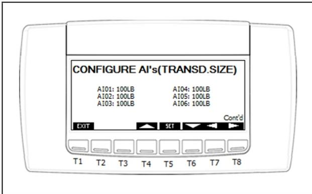
Figure 9-7 - Configure Analog Input's Transducer Size
