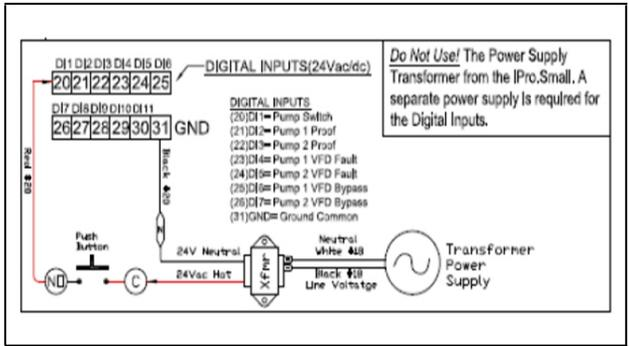
Figure 4-4 - Digital Input Wiring - 31 GND is Digital Common -
