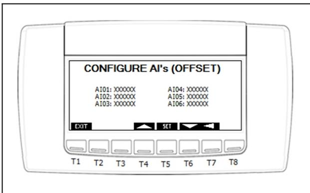
Figure 9-8 - Configure Analog Input's Offset
