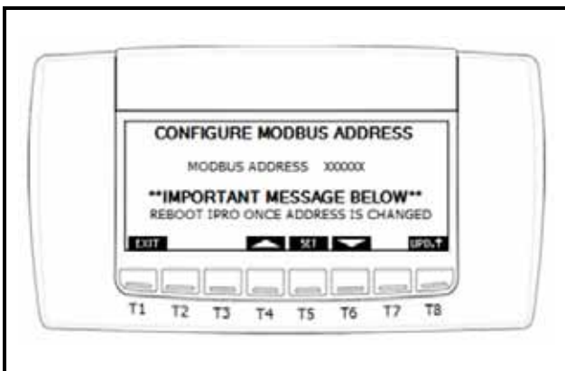
Figure 9-18 - Configure MODBUS Address
