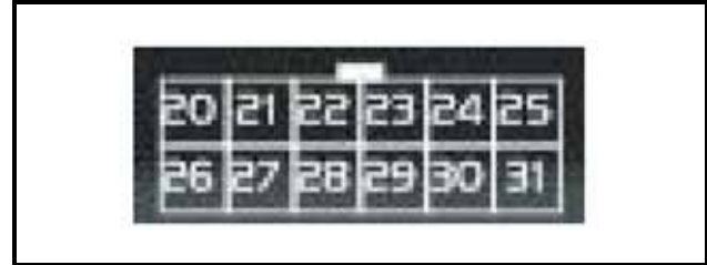
Figure 4-5 - Digital Input Connectors
