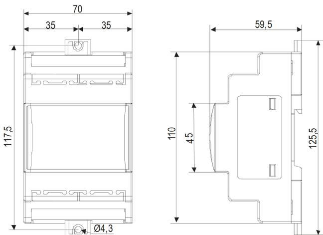
EXD-SH1/2 are stand-alone universal superheat and or temperature controllers for air conditioning units or refrigeration systems.
