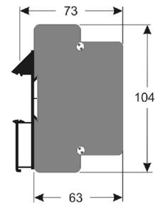
**EC3-P32 / -P33** are stand-alone universal superheat controllers. **EC3-P32** offers remote access with built-in TCP/IP Ethernet communications and WebServer functionality. Any standard WebBrowser (e.g. Internet Explorer or Mozilla Firefox) can be used for monitoring or parameter setting. **EC3-P33** has no network communication.
