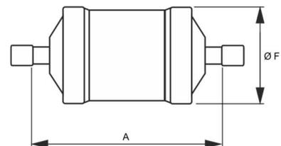
BFK-...FLR filter-driers are used for protection of systems against contaminant.
