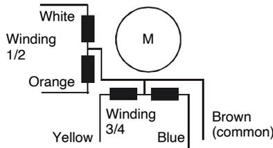
**EXM-24U/EXL-24U (24 VDC, 5 wires coil)**
