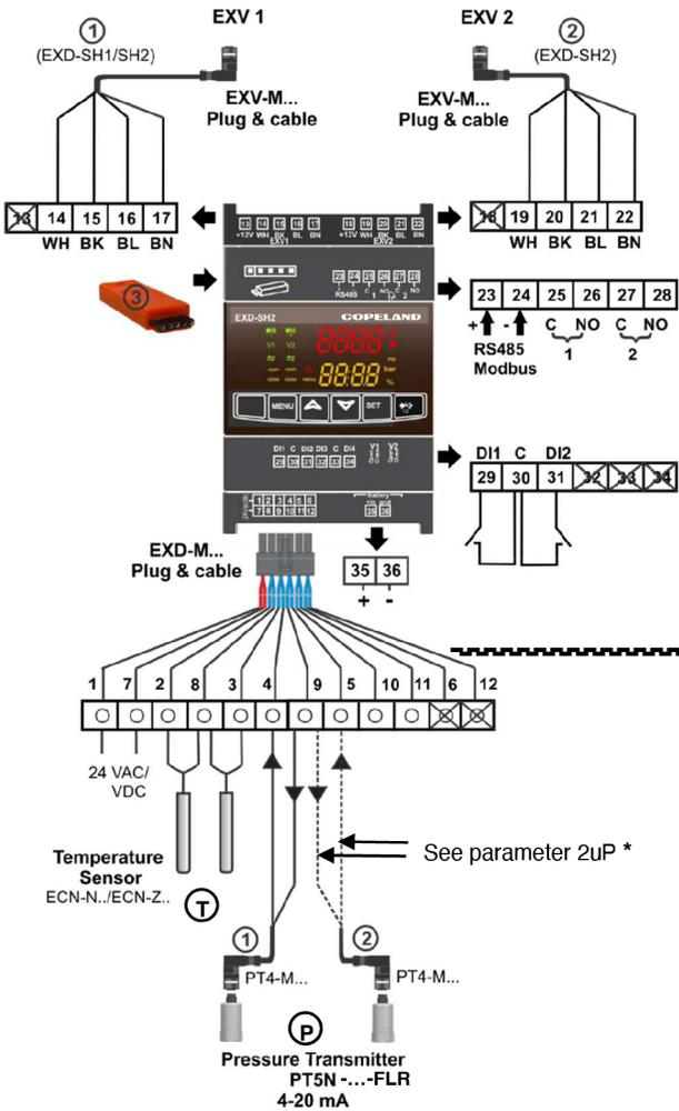
Wiring options: UPS (ECP-024)/Supercap (EXD-PM)
