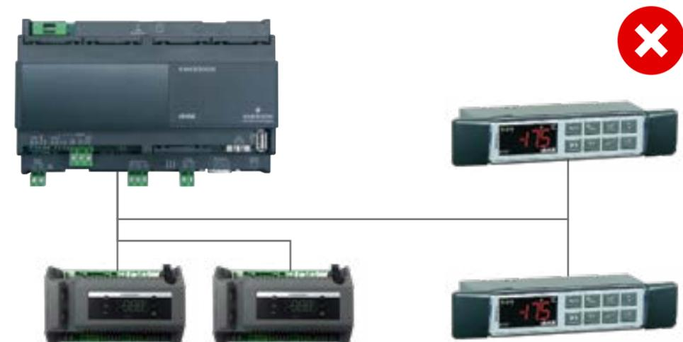
Figure 10. Incorrect network wiring
