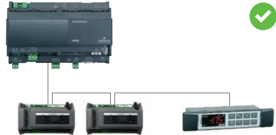
Figure 9. Correct network wiring
