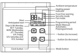
The programmable thermostat has three main operating modes: Manual (**man**), Automatic (**AUTO**) and Preprogrammed (**PRE-PROG**). The active mode is displayed at the bottom of the screen. The transition from one mode to another is done by pressing down the **MODE**, button, out of any adjustment mode.
