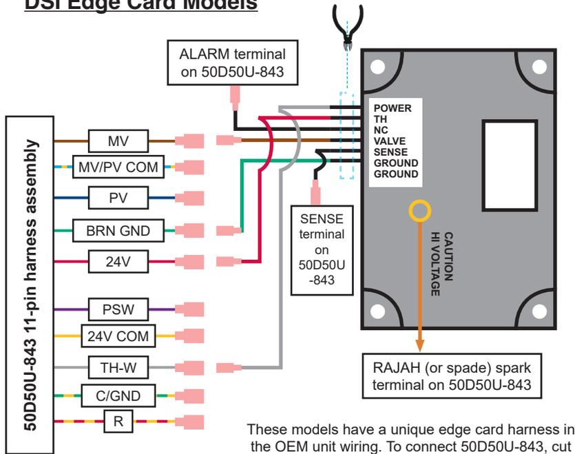
These models have a unique edge card harness in the OEM unit wiring. To connect 50D50U-843, cut each individual wire from the edge card harness, attach 1/4" QC spade terminal and connect directly to 11-pin harness.
