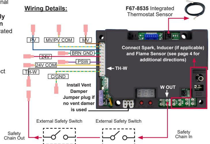
**IMPORTANT: Connect W Out on 50D50U-843 module to input of safety switches (limit, rollout, etc.) and connect output of safety switches to TH-W on 50D50U-843**
